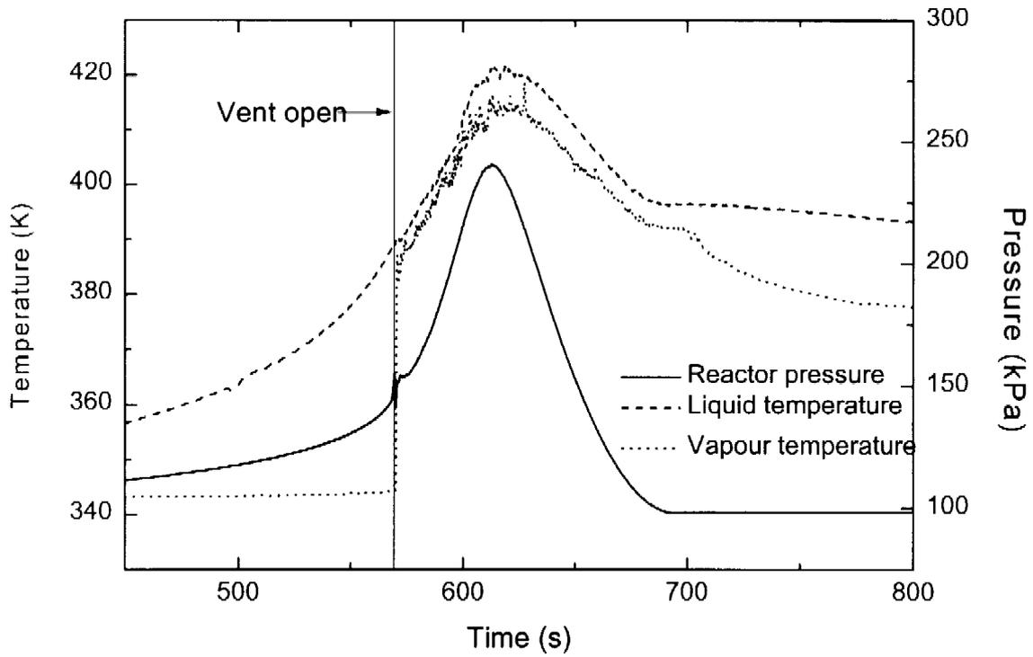
FIGURE 5 Reactor temperature and pressure records for a gassy systems
