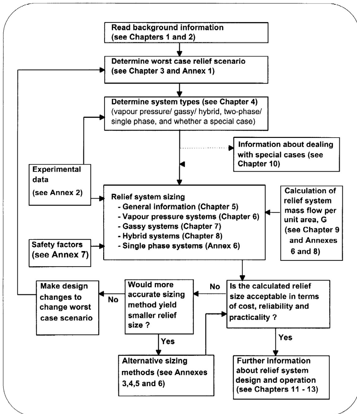
FIGURE 2 Steps in the design of a relief systems for a runaway chemical reaction
